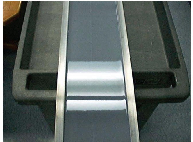
Finished epoxy surface on calibration beam reflecting the overhead fluorescent lighting fixture. Image courtesy of Phoenix Scientific Inc.
